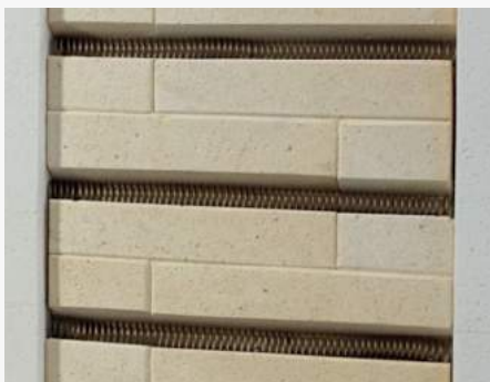
Heating elements in grooved bricks
