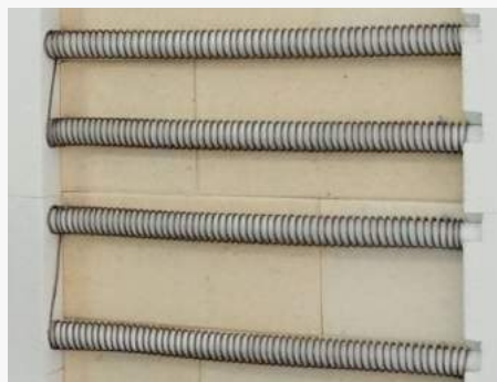
Heating elements on support bars
