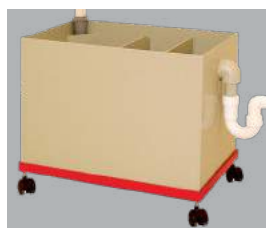
✓ Devices: Sedimentation tanks
